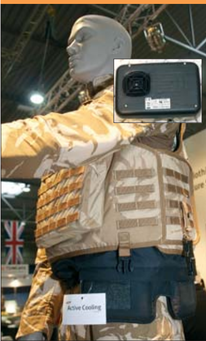
The infantry version of the Gore Active Cooling (the black element) is worn under a body armour. Following trials in operational theatres the company is discussing honing the latest details before starting production. The fan (inset) is in the lower pocket of the garment. (Armada/PV)
