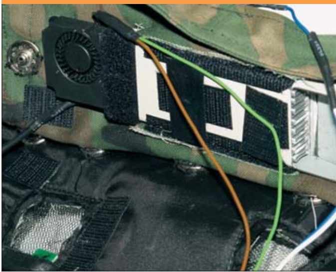
The Pelletier cell and the blower of the Gathergy liquid circulated cooling system are more complex than air blown cooling vests; the advantage of such a system is that it is possible to set the desired temperature. (Armada/PV)
